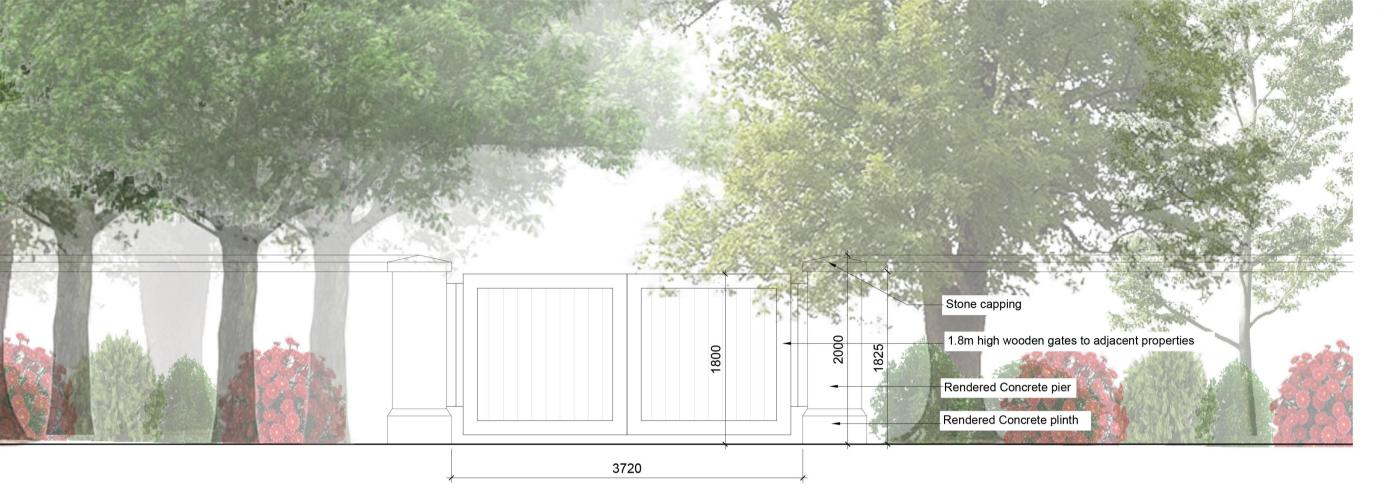
PROPOSED GATES ELEVATION FROM APPLICANT'S SIDE - GATES TO ADJACENT PROPERTIES IN STREAMSTOWN SCALE 1:40
